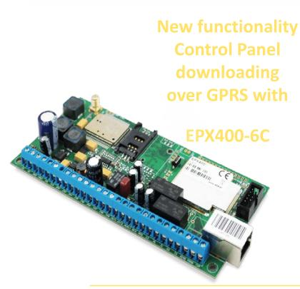
Transmitter based on LX20G5C, providing extended functionality. This specifically includes remote configuration of the LX20G-5C together with configuration of other control panels - novel features of EBS products. It allows the client to **reduce the cost** of installing and configuring the unit, but also improves services and technical inspections.
